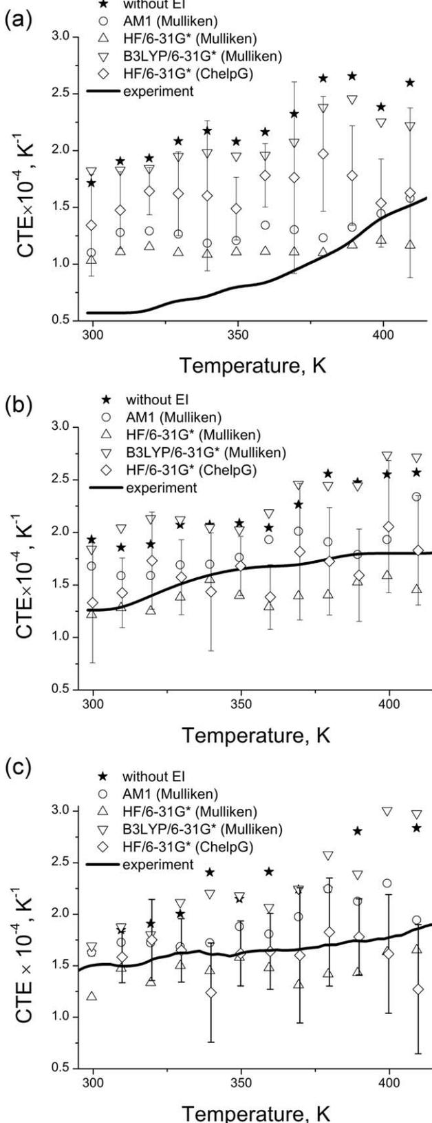
**FIGURE 2** Temperature dependences of CTE for R-BAPS (a), R-BAPB (b), and R-BAPO (c) PIs with EI parameterized by AM1(Mulliken) (open circles) HF/6-31G\* (Mulliken) (open triangles), B3LYP/6-31G\*(Mulliken) (open inverted triangles), HF/6-31G\*(ChelpG) (open diamonds) methods and without EI (black asterisks). Experimental CTE values are shown by black solid curves. Typical values of error bars are shown for HF/6-31G\*(ChelpG) method.
