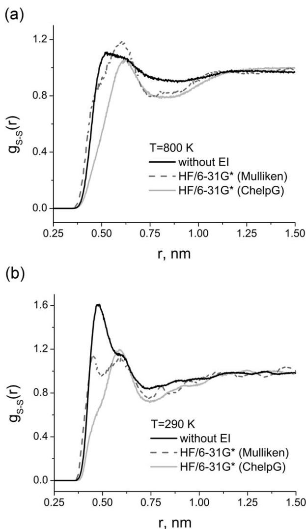
**FIGURE 5** Pair distribution function  $g_{s-s}(r)$  calculated between sulfur atoms for PI R-BAPS at  $T=800$  K (a) and  $T=290$  K (b) without EI and with EI parameterized by HF/6-31G\* (Mulliken) and HF/6-31G\*(ChelpG) methods.
