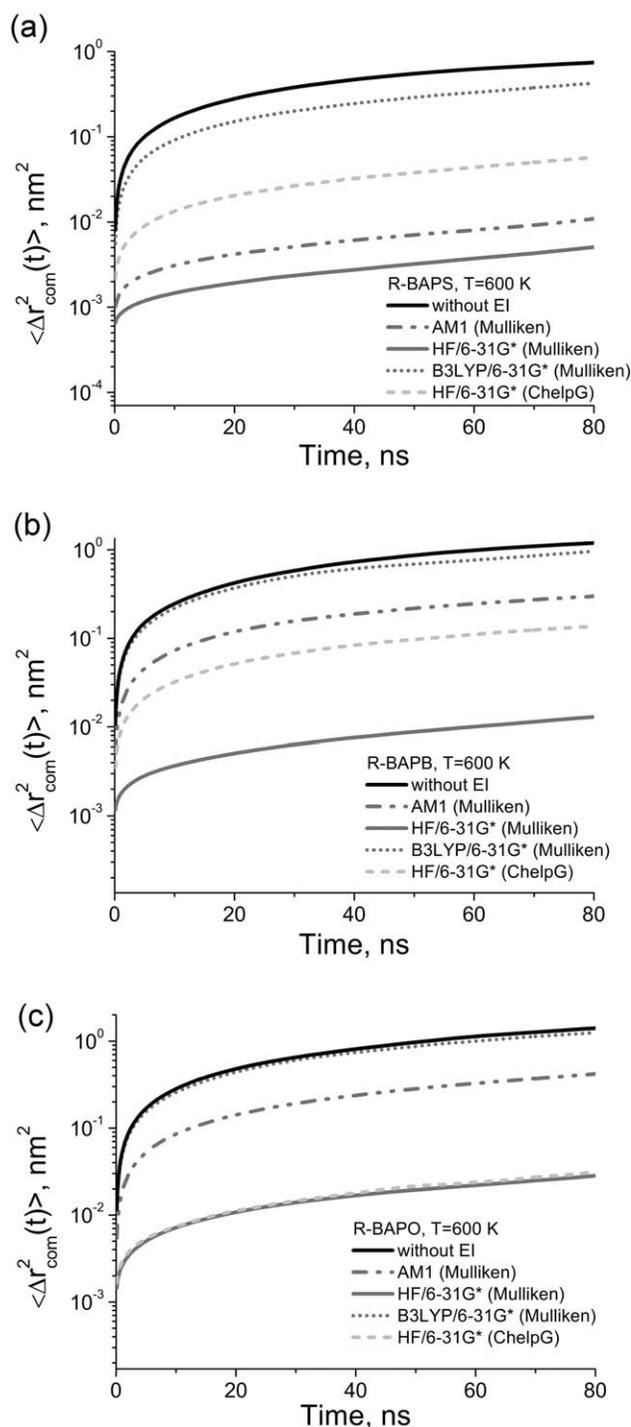
**FIGURE 3** Time dependence of the mean square displacement  $\langle \Delta r_{\text{com}}^2(t) \rangle$  for the center of mass of R-BAPS (a), R-BAPB (b), and R-BAPO (c) PIs chain with EI parameterized by AM1 (Mulliken) (gray dashed line), HF/6-31G\* (Mulliken) (gray solid line), B3LYP/6-31G\* (Mulliken) (gray dotted line), HF/6-31G\* (ChelpG) (gray dash-dot line) methods and without EI (black solid line)
