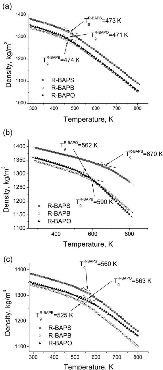
**FIGURE 4** Temperature dependences of the density for three PIs under investigation during the cooling procedure from 800 to 290 K without EI (a) and with EI parameterized by HF/6-31G\*(Mulliken) (b) and HF/6-31G\*(ChelpG) (c) partial atomic charges. The error in the calculated  $T_g$  values for all investigated PIs obtained with all three indicated EI parameterizations was  $\sim 8$  K.
